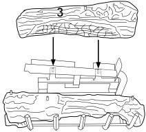
Figure 47 - Installing Log No. 3
